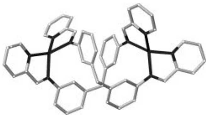
Figure 1. View of the cation [\text{Cu}_2(\text{L}_a)_2]^{2+} , the copper coordination sphere is shown in black.
